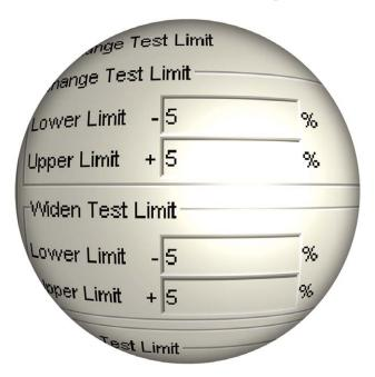
Available in the graphical debug interface introduced at software version 07.00 for the Agilent Medalist i3070 test system, the Auto Optimizer is a tool designed to automatically evaluate and fine-tune analog in-circuit tests in order to improve throughput.
